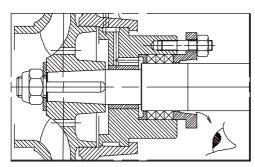
If the pump has a packed gland there must be some leakage from the gland. Gland nuts should initially be finger tight only. Leakage should take place soon after the stuffing box is pressurized. If no leakage takes place the packing will begin to overheat. If overheating takes place the pump should be stopped and allowed to cool before being restarted. When the pump is restarted it should be checked to ensure leakage is taking place at the packed gland.
